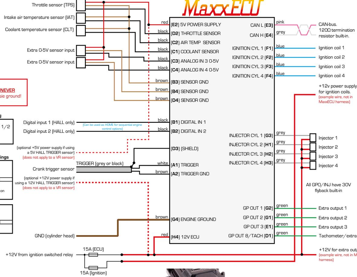
Sensor GND must **NEVER** be connected to chassis ground!
