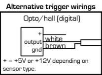
(optional +5V power supply if using a 5V HALL TRIGGER sensor) (does not apply to a VR sensor)
